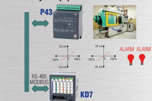
**Measurement and displaying of the network parameters and energy of the 3-phase machines**
